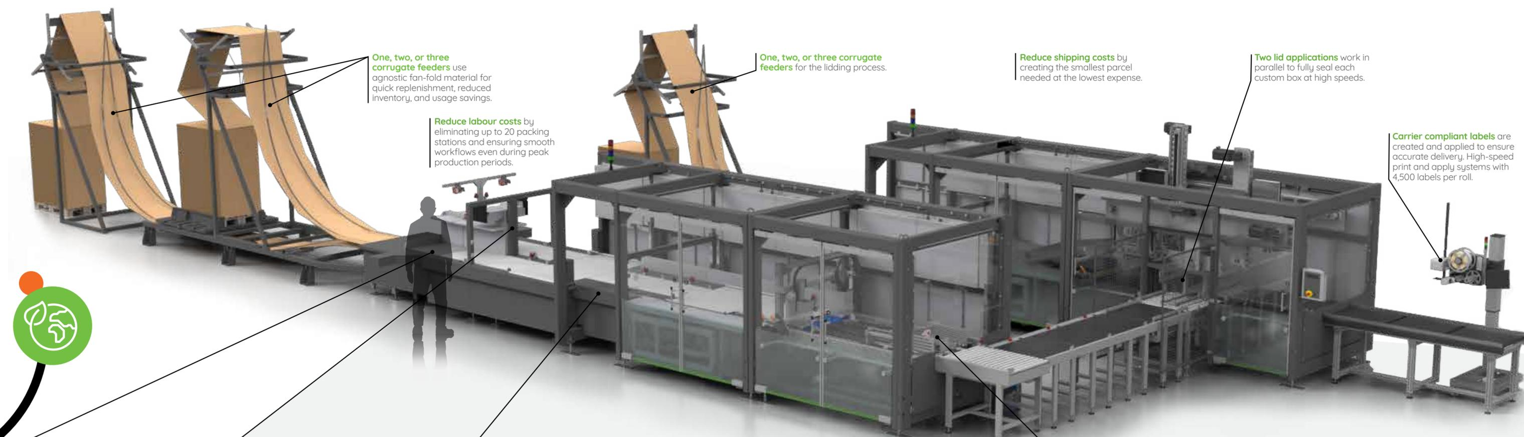
**One, two, or three corrugate feeders** use agnostic fan-fold material for quick replenishment, reduced inventory, and usage savings.
